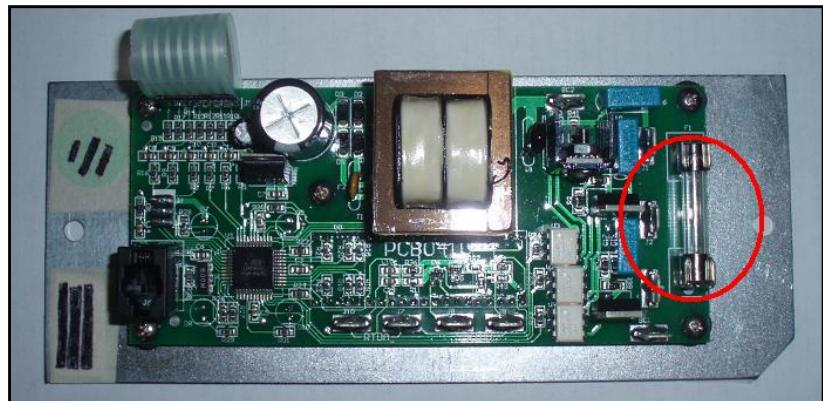
\*European models use a 1-1/4" x 1/4", 5 Amp, 230 Volt Fast-Blow Cartridge Fuse
